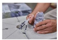
In Ghassemi's Rock Mechanics Lab, rocks are put to a variety of tests to determine their characteristics and response to injection. Ghassemi holds a core sample with a natural fracture that was tested with acoustic emission (seismicity) monitors used in the testing.
