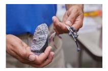
In the Rock Mechanics Lab, researchers can study the relationship between the noise rock makes (micro-seismicity) and its flow capacity increase. Acoustic emission monitors like these record noises related to sliding of fractures, and are correlated with permeability increase.
