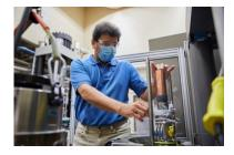
Ghassemi inserts a core sample into a machine that will simulate the pressure of rocks deep in the earth.
