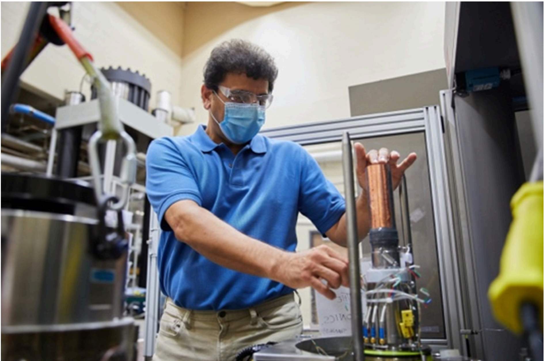
In Ahmad Ghassemi's Rock Mechanics Lab, rocks are put to a variety of tests to determine their characteristics. Ghassemi inserts a core sample into a machine that will simulate the pressure of rocks deep in the earth.
