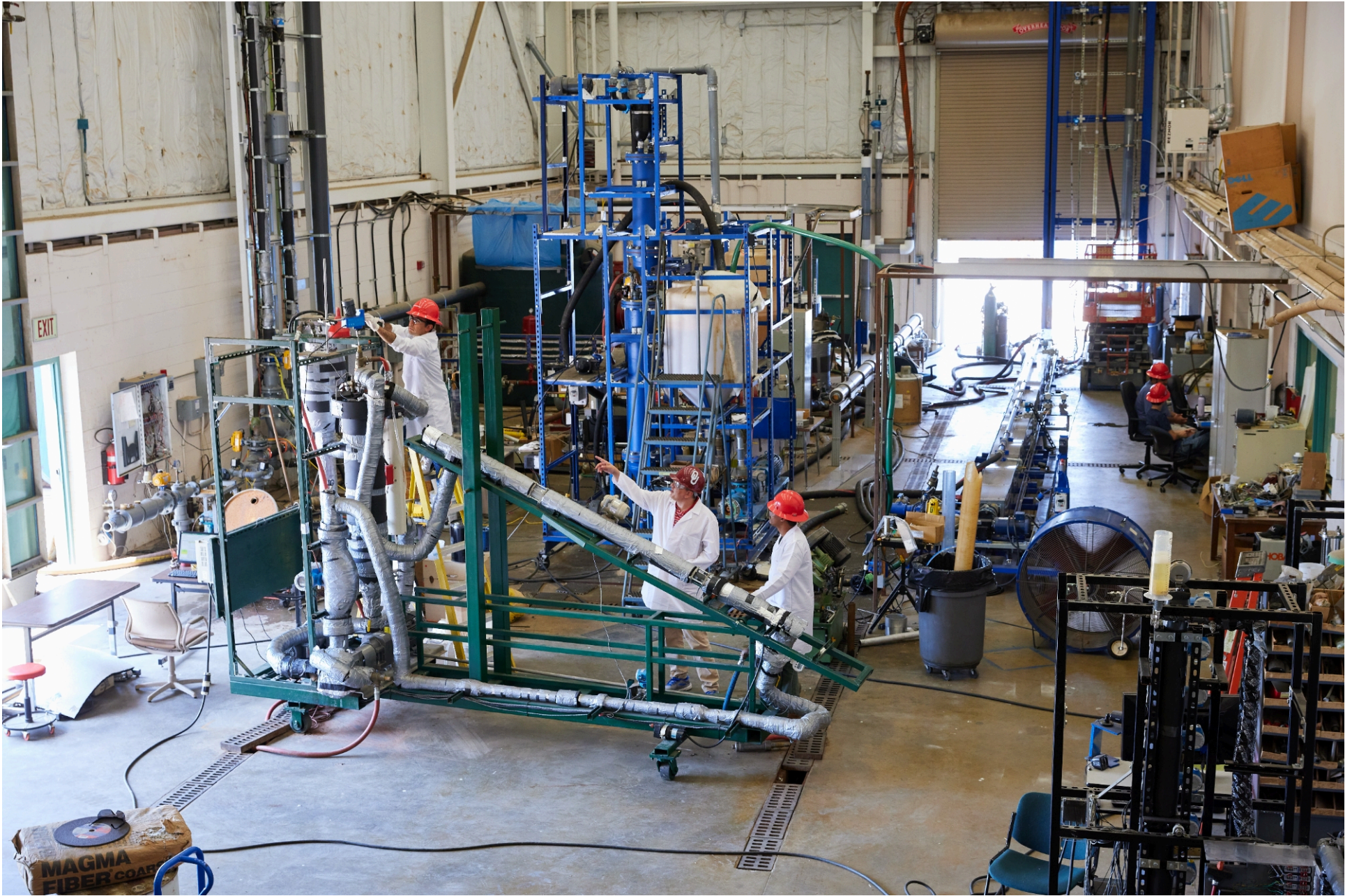
At the Mewbourne School of Petroleum and Geological Engineering's one-of-a-kind Well Construction Technology Center at OU's north campus, Ph.D. students Cesar Vivas (left) and Majeed Mohamed (right) are helping Salehi (center) to conduct experiments on a geothermal flow loop used for investigating suitable fluids for drilling hot geothermal formations. Image by Travis Caperton.
